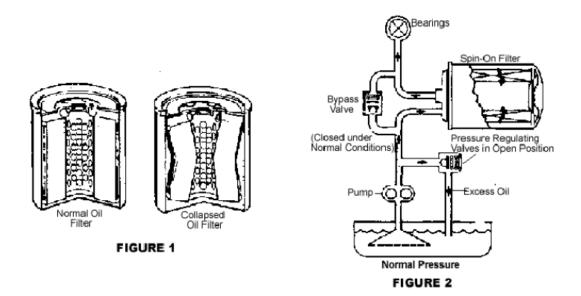
Oil filters are designed to withstand, without collapsing, differential pressures significantly greater than those experienced under normal operating conditions.
